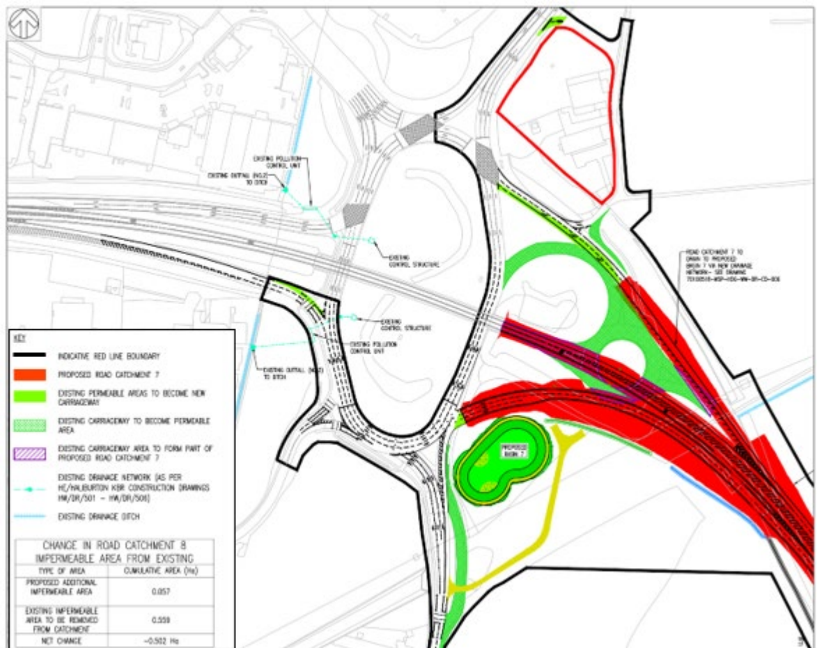
Figure 7-1 – Hardwick junction drainage/catchment 8
