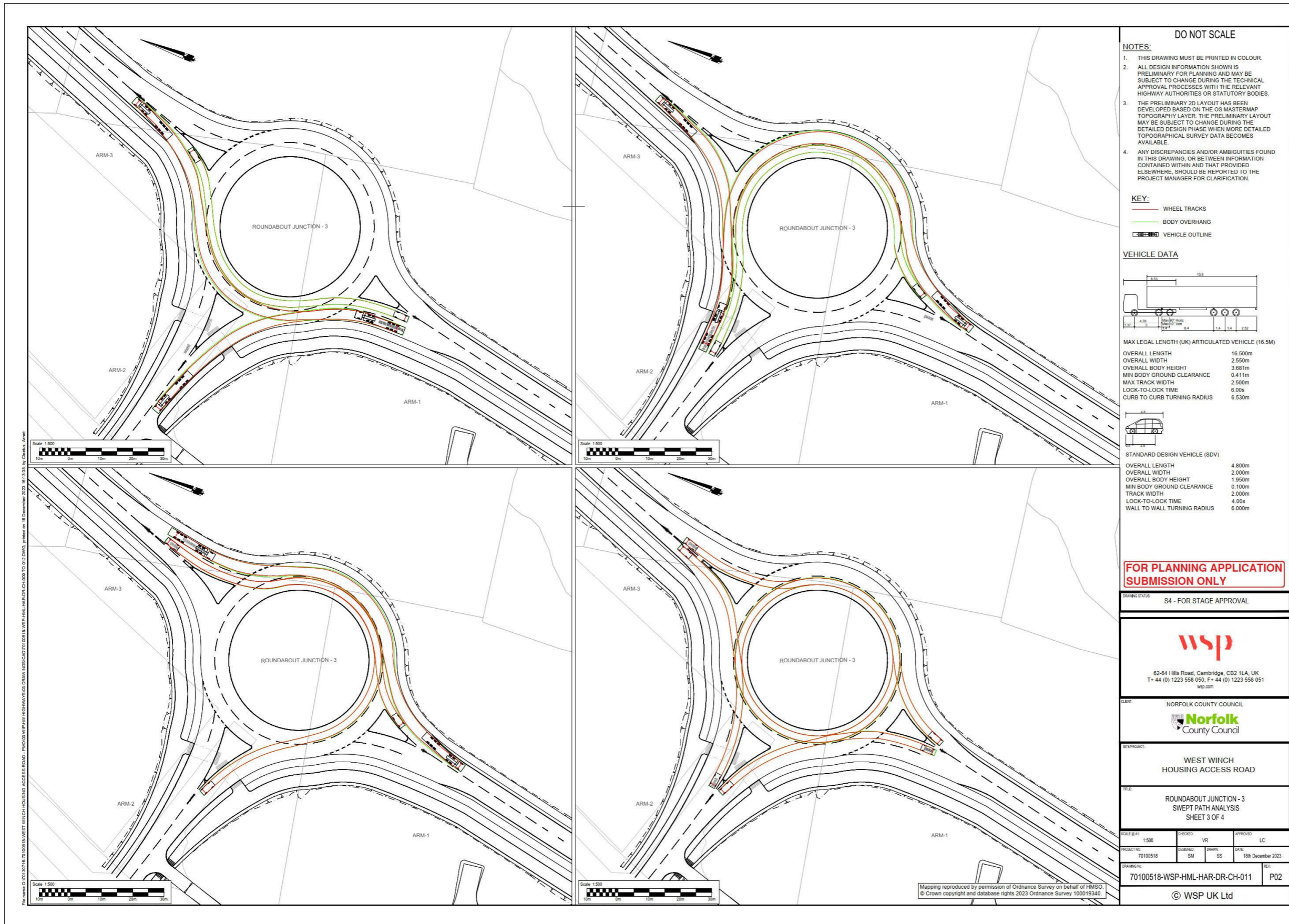
Figure 6- Swept Path for HAR (Sheet 3 of 4)
