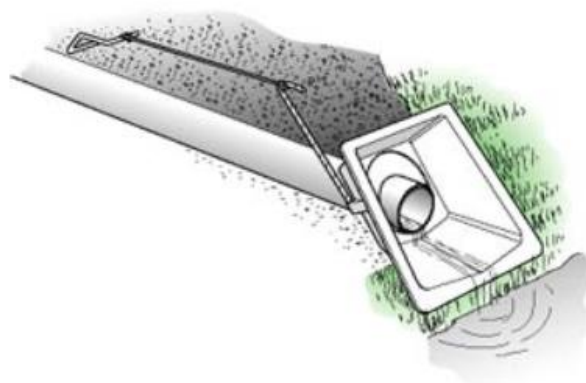
Figure 6-4 General purpose headwall unit
