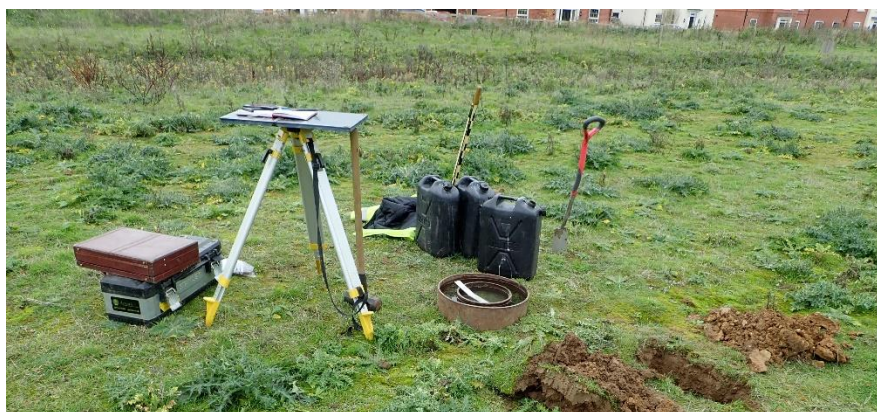
Figure 4-2 Infiltration rate measurement on the site
