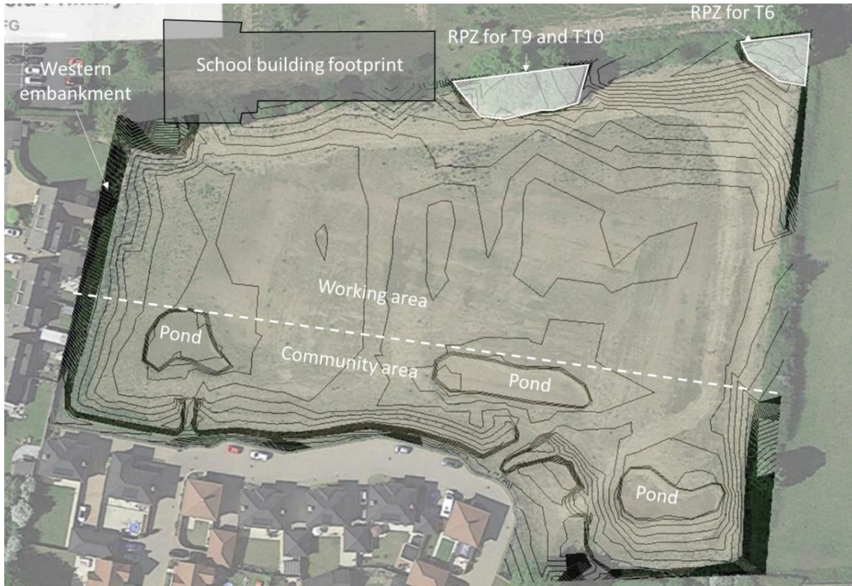
Figure 3-6 Existing topography with key feature annotations
